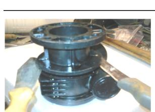
Use 2 knifes or flat screw drivers to push the flang of. Do the same with the cover on the other side. Finish one side before you take the next one.
